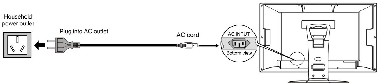
1. Connecting the female plug to the AC socket on the unit.
